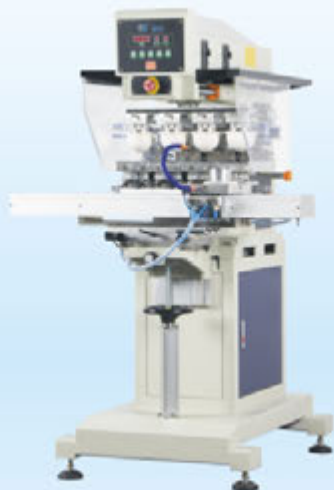
SP-858SD 氣動五色穿梭移印機 Pneumatic 5-color pad printer with shuttle
