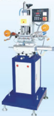
H-250S 氣動平面/曲面燙金機 Pneumatic Flat/Cylindrical Hot Stamping Machine
