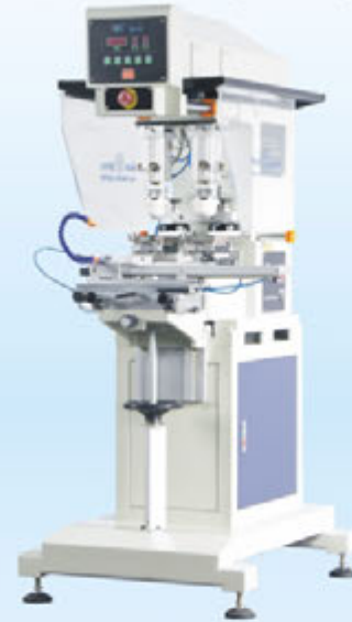
SPCS-848SDQ1 獨立印頭伺服穿梭四色移印機 4Color Pad Printer with Independent Pad Stroke and Servo Shuttle
